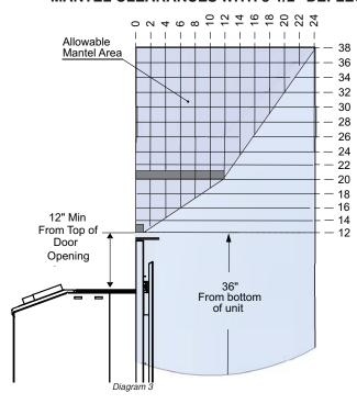
Note: A 3-1/2" mantel deflector to reduce mantel height to 36" from bottom of unit @ 1"depth.
